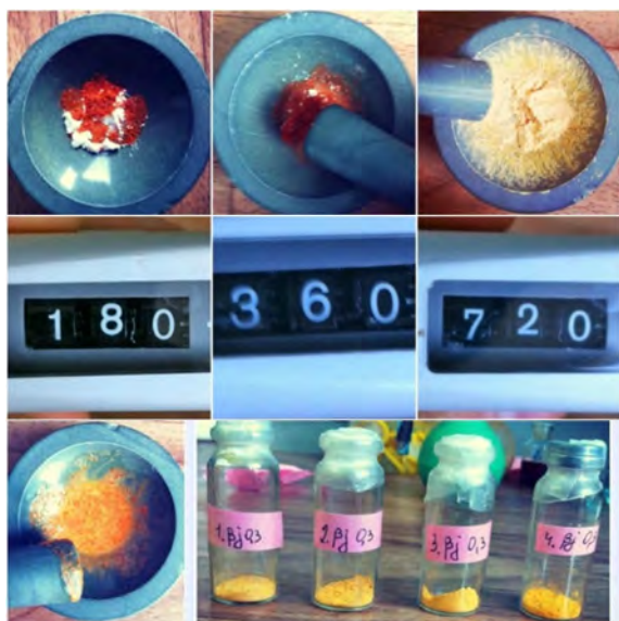
Figure 2. Obtaining binary systems (juglone and \beta CD) by the kneading method.
