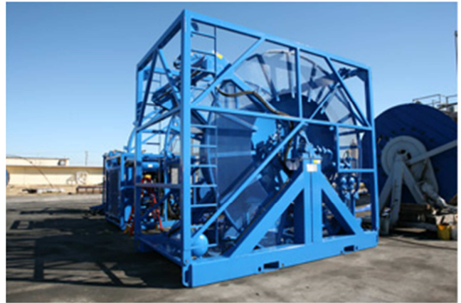
Figure 8. Coiled tubing reel, 22,000 ft. to 2 inches [13].
