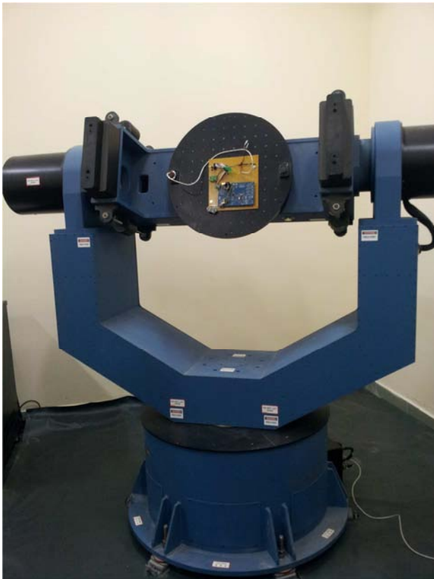
Figure 8. Test on the turntable three degrees of freedom.
