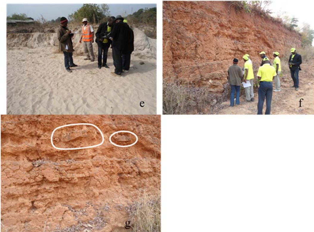
Figure 8. Geological mapping in the Bida Basin; (e) Loose sands of the Enagi Formation at the village of Batati on the Bida-Mokwa road; (f, g) Concretionary ellipsoidal ironstone in clayey groundmass of Batati Formation at Pattishabakolo near Bida.
