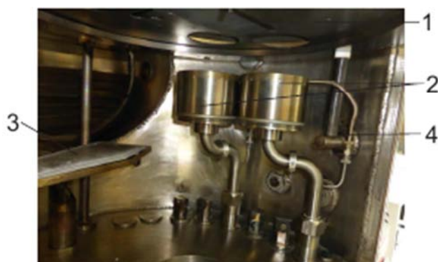
Figure 2. Device beneath the lid of VU – 1A-type vacuum machine with two modernized magnetron sputtering sets. 1 – disk-shaped horizontal carouse, 2 – magnetron sputtering device with Si and Zr targets, 3 – lens concentrator cleaning device, and 4 – O_2 and Ar individual gas flow system, directly connected to magnetron sputtering device.
