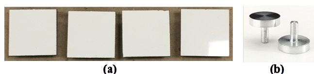
Figure 4. Image of (a) sample to be tested and (b) aluminum sample holder
