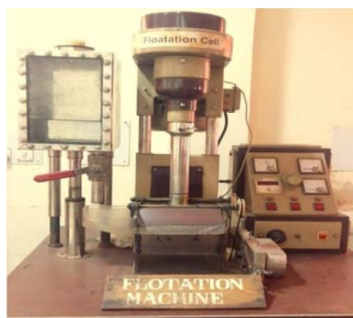
Figure 1. Scheme of Laboratory flotation cell.
