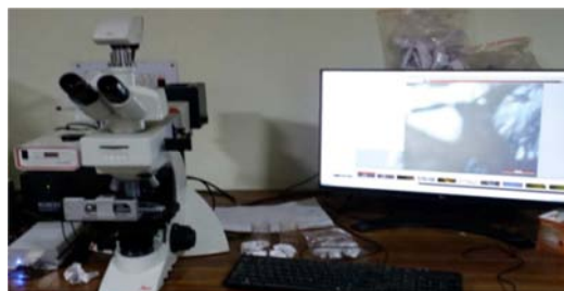
Figure 2. Petrographic set-up attached with an oil immersion lens connected to computer.
