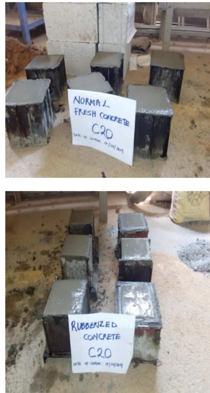
Figure 3. Casting of control and rubberized concrete specimens.
