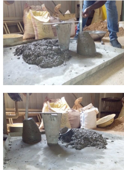
Figure 2. Slump of normal and Rubberized Concrete.
