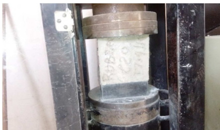
Figure 8. Rubber reinforced concrete and normal concrete exhibiting some cracks after being subjected to heat at 100°C for 48 hours.
