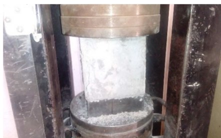
Figure 9. Compression test of heated rubber reinforced concrete.
