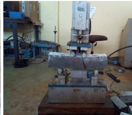
Figure 4. Center point loading flexural strength test.
