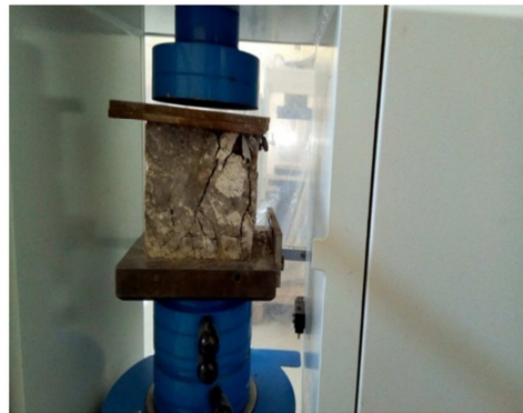
b. Fiber reinforced concrete cube sample after test
