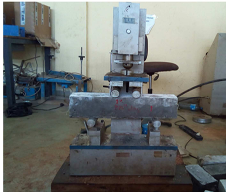
Figure 4. Center point loading flexural strength test.
