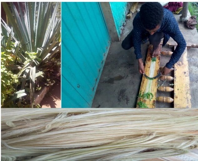
Figure 1. Sisal plant, and beaten by a knife and removing excess amount of waste and sundried sisal fiber in 50 mm.
