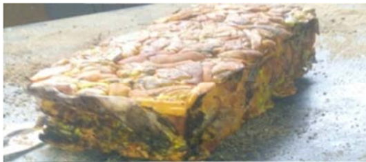
Figure 3. Produced HDPE Plastic Brick.
