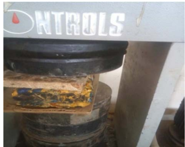
Figure 4. Compressive Strength Test for Plastic Brick.
