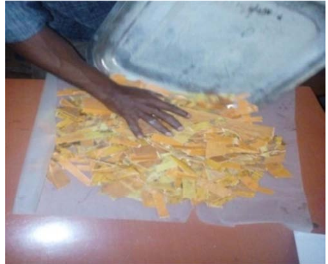
Figure 1. Reduced Size of High-Density Polyethylene (HDPE).
