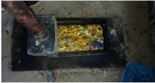
Figure 2. Compaction of Melted HDPE Plastic Waste in Mould.
