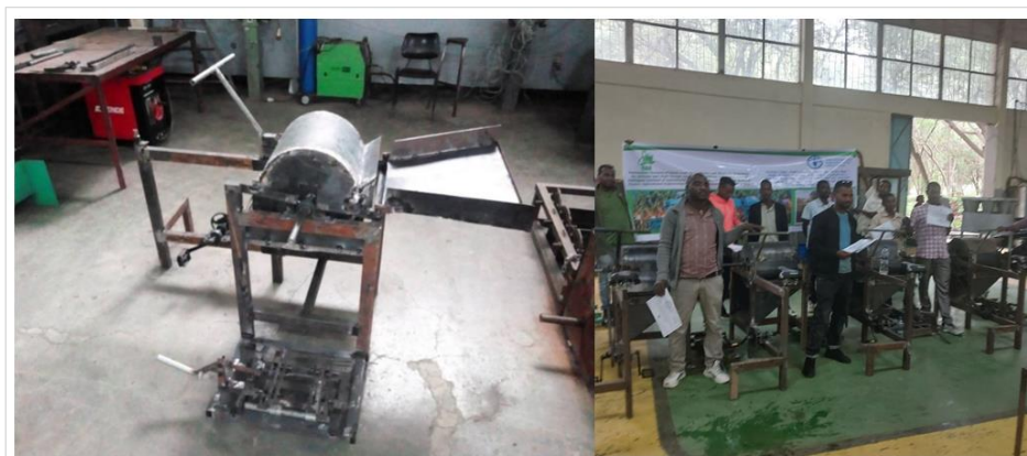
Figure 5. Final prototype of maize sheller Fabricated by artisans.
