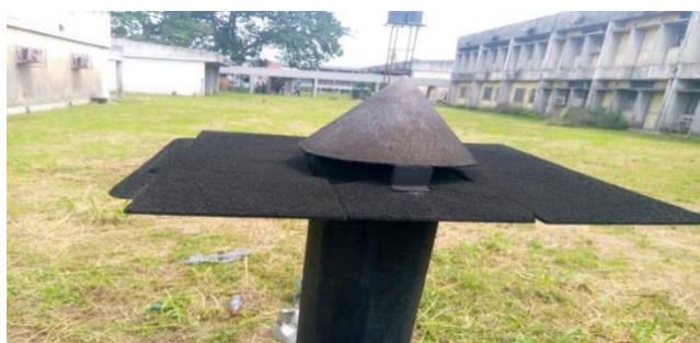
Figure 2. Deposition of Fly Ash on Tray during Sample Incineration.
