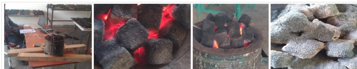
Figure 2. Procedure of Carbonized Rice Husk Briquetting burning from starting and final stage.
