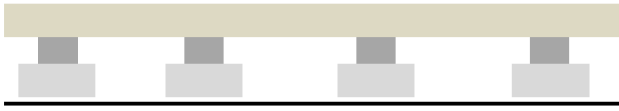
Figure 5. System analysis is done considering all LRBs as horizontal springs placed parallelly.
