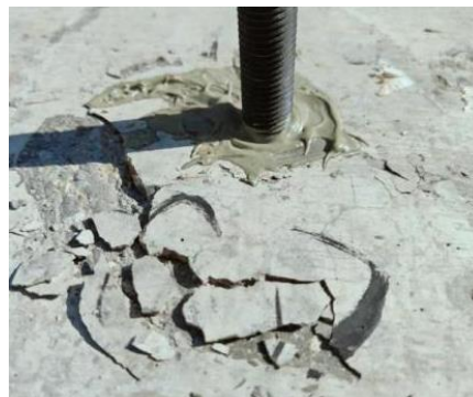
Figure 1. Diagram of anchor bolt pull-out failure.
