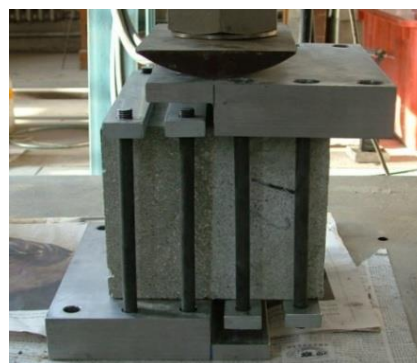
Figure 2. Direct shear test setup.
