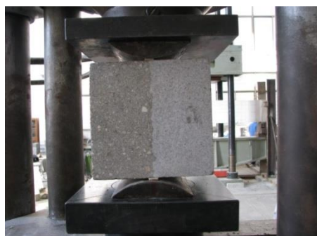
Figure 1. Splitting tensile test setup.
