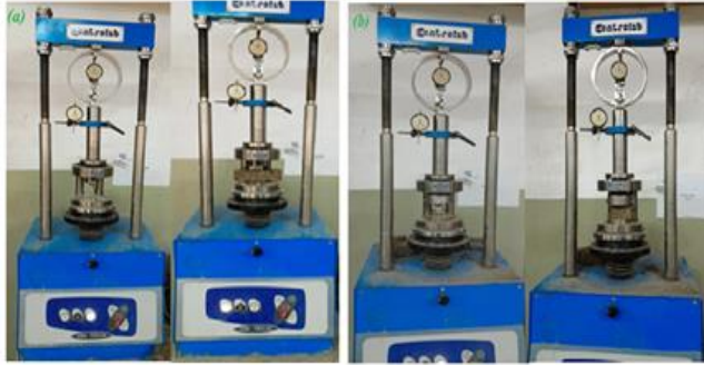
Figure 2. CBR press with different three-point bending and single compression cells.
