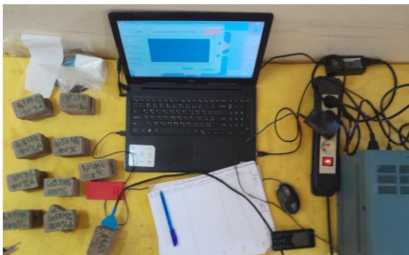
Figure 3. FP2C conductivity meter with its accessories.
