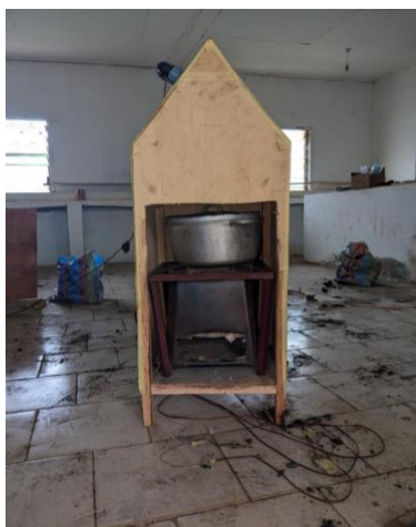
Figure 2. Water boiling testing setup.
