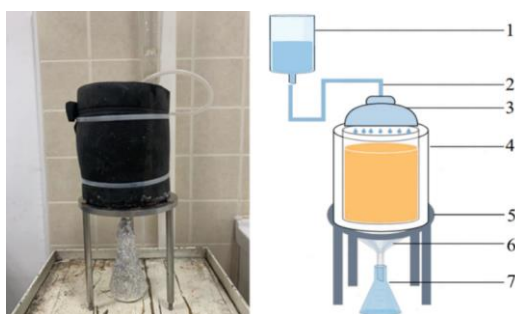
Figure 2. Physical picture and structural diagram of the leaching simulation device(1- Water storage bottle, 2- latex tube, 3- nozzle, 4- acrylic column, 5- rack, 6- funnel, 7- conical flask).
