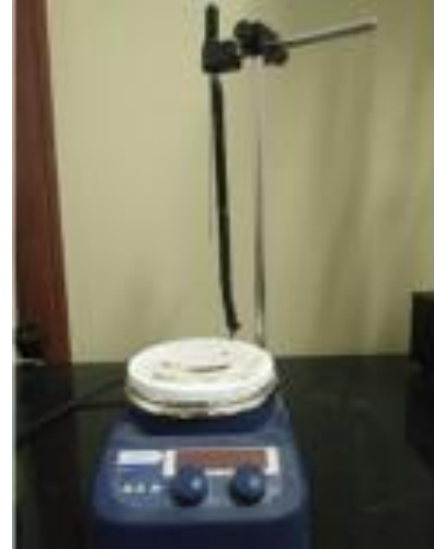
Figure 2. The magnetic stirrer to the mixed polymer is used for determining fracture toughness.
