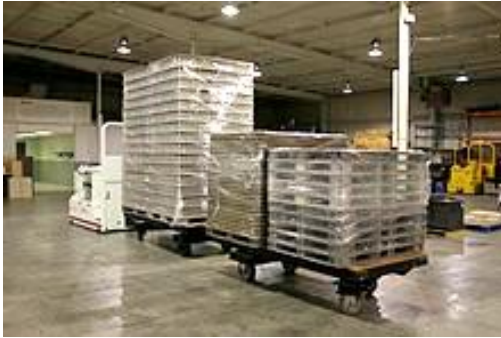
Figure 3. Tugger AGV towing multiple trailers in a warehouse environment. (Wikipedia).
