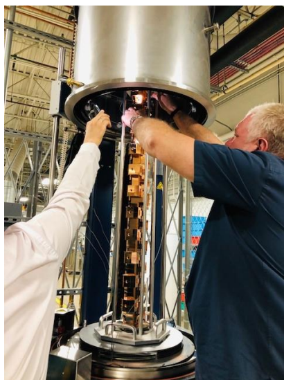
Figure 19. ABC-9-S-O-X-T being set in a brazing furnace.
