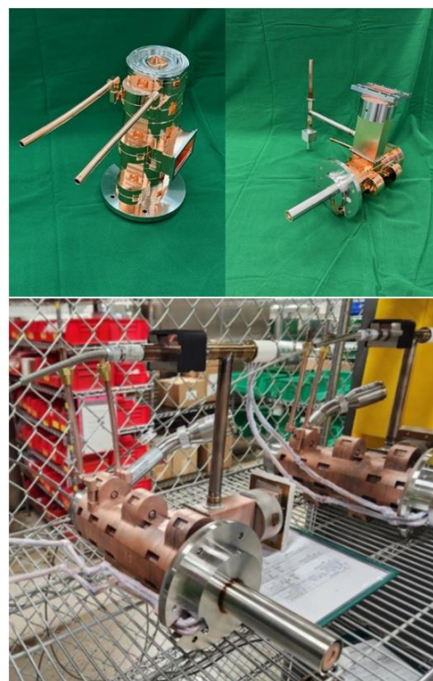
Figure 15. ABC-6-S-M-X In order as shown: Final Braze Assembly (1) Vacuum Assembly ready for vacuum processing (2); Completed, ready to ship ABC-6-S-M-X-D (3).
