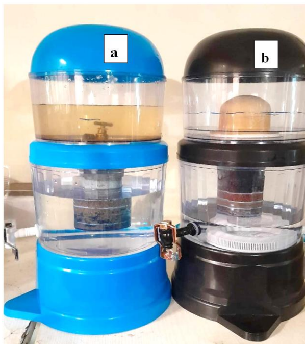
Figure 6. View of the designed filter (Intermittent Bio sand filter) in (a) and the control filter (ceramic filter) locally found on the market in (b).
