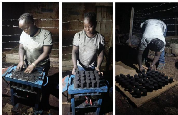
Figure 9. Compaction operation ecological charcoal briquettes obtaining.
