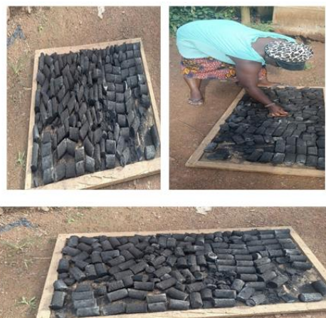
Figure 10. Briquettes final drying.
