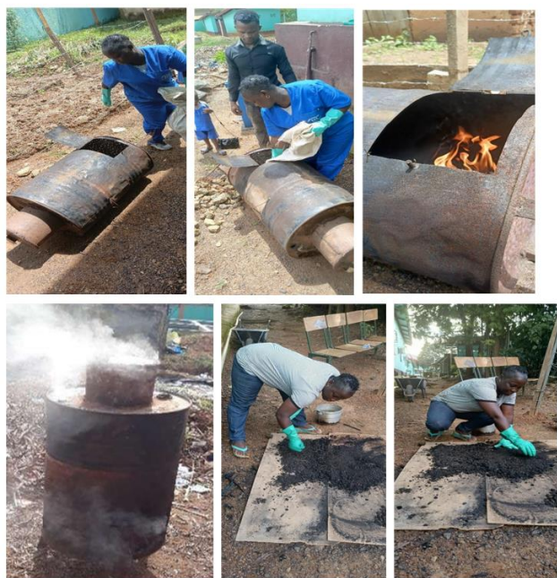
Figure 5. Carbonization operation.
