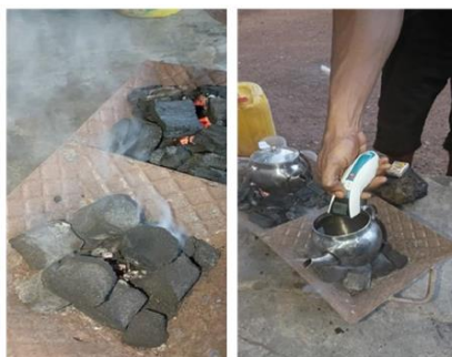
Figure 12. Combustibility test: comparison between wood charcoal and ecological charcoal produced from pig manure.
