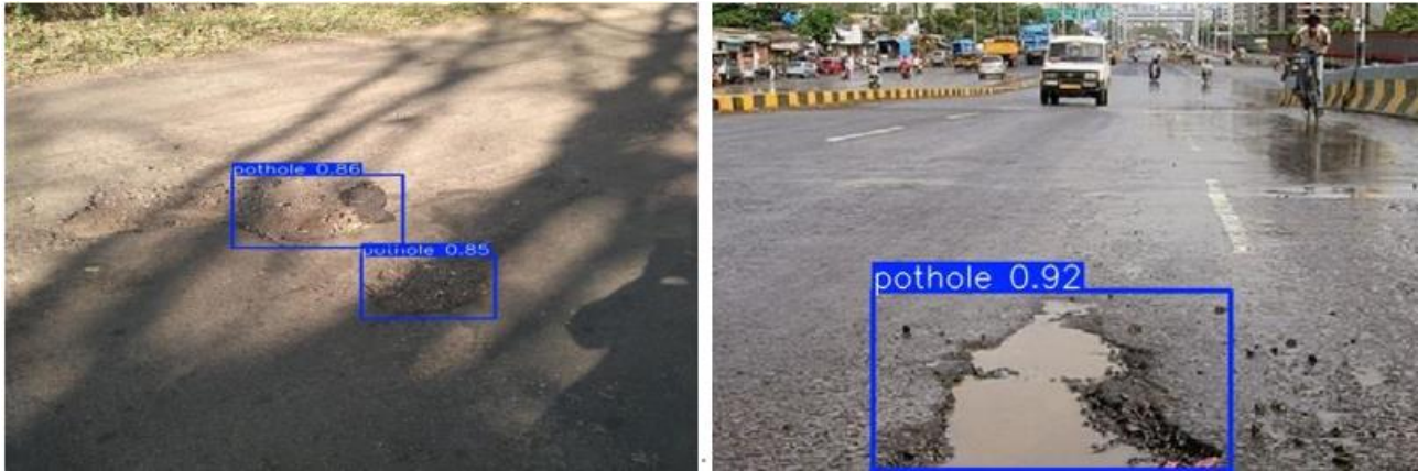
Figure 4. Sample Pothole Detection Results on Test Images.
