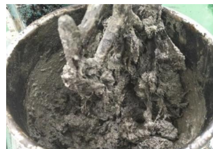
Figure 2. Emulsified Asphalt Demulsified after Mixing with Cement and Lost Workability.
