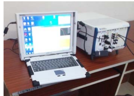
Figure 3. NI PXIe VST based Set-up for LTE.
