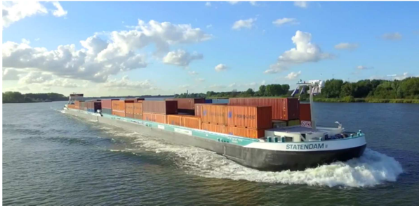
Fig. 1. Statendam I and II, a double propeller inland vessel with a hybrid propulsion system.
