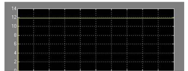
Figure 9. Output voltage of fuzzy controlled buck converter for 20 supply voltage.
