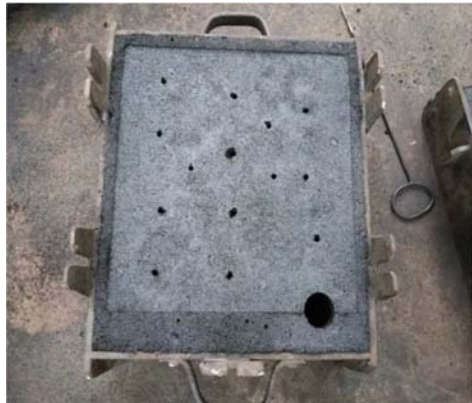
Figure 5. Molasses preparation for mold making.
