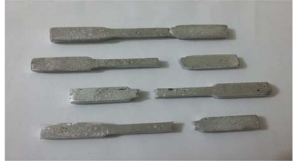
Figure 8. Samples after tensile testing.
