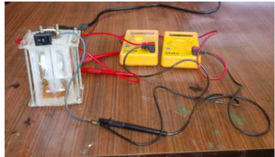
Figure 8. Experimental setup for Measuring Voltage and Current.
