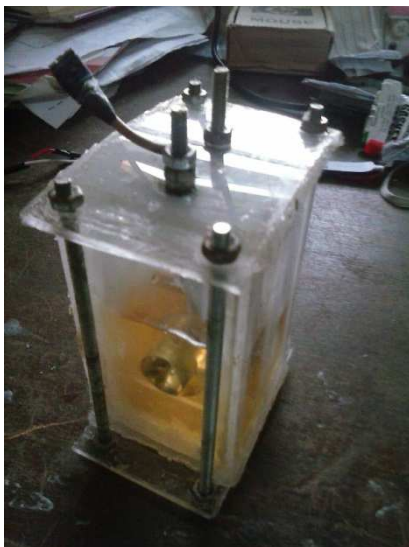
Figure 7. The constructed hydrogen fuel cell.
