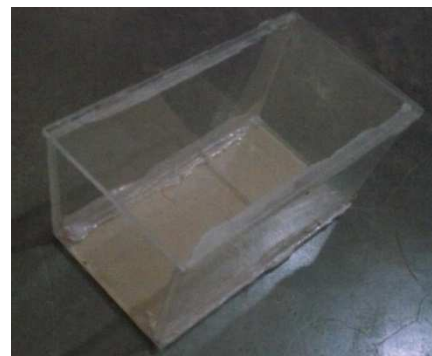
Figure 4. Outer case development for the fuel cell.
