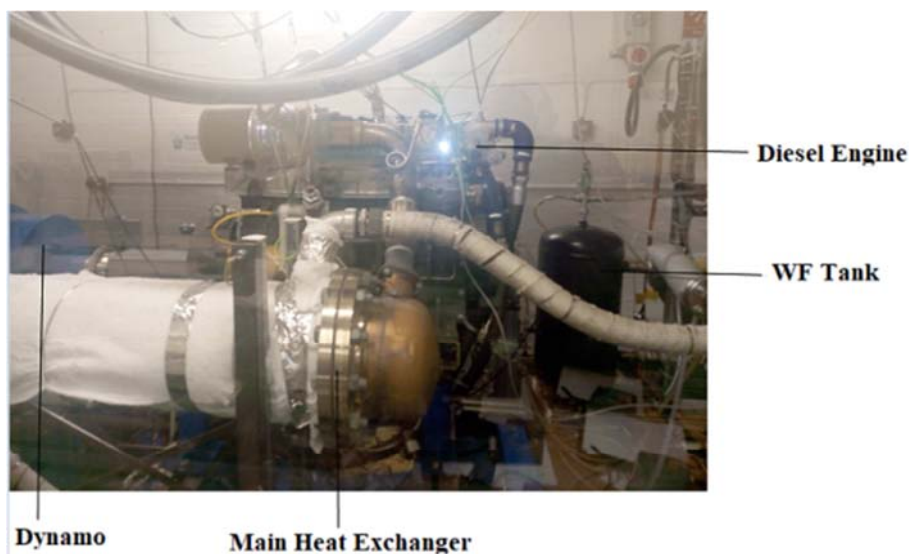
Figure 2. Primary Components of the Test-bench.
