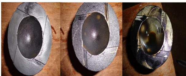
Figure 2. Piston crown surfaces showing slots of widths.
