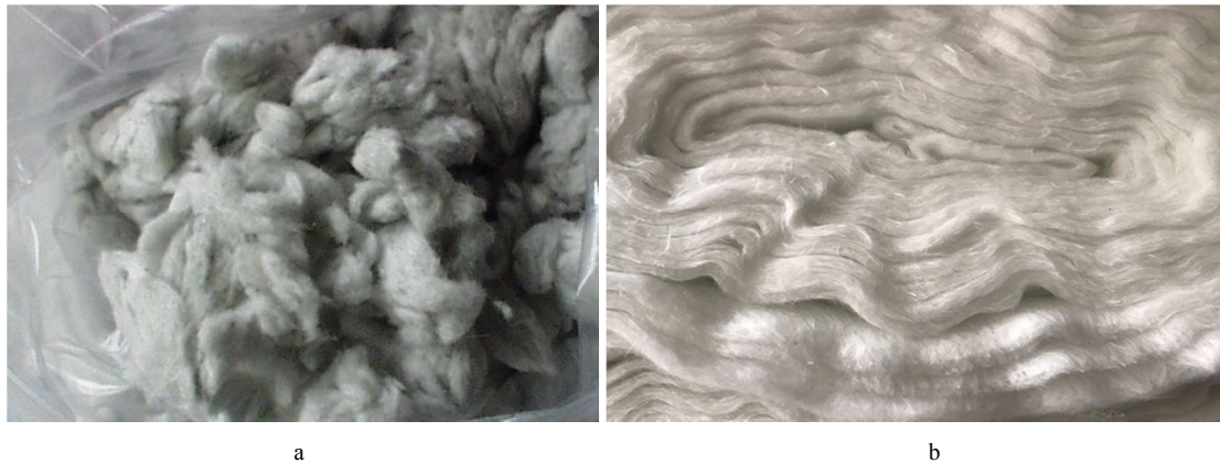
Figure 1. a: the digital photo of rock wool; b: the digital photo of glass wool.
