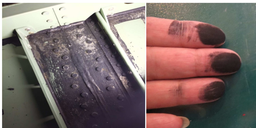
Figure 3. Sealing glue layer in the fuel tank of an aircraft after 1000 flight hours.
