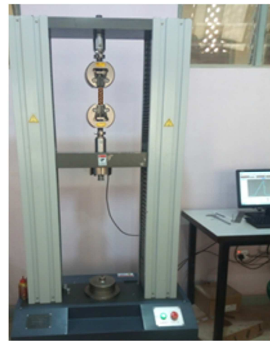
Figure 3. Instron Tensile Testing Machine Used to Tests the Composite Laminates.
