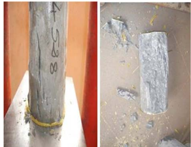
Figure 4. Samples after compressive strength test.
