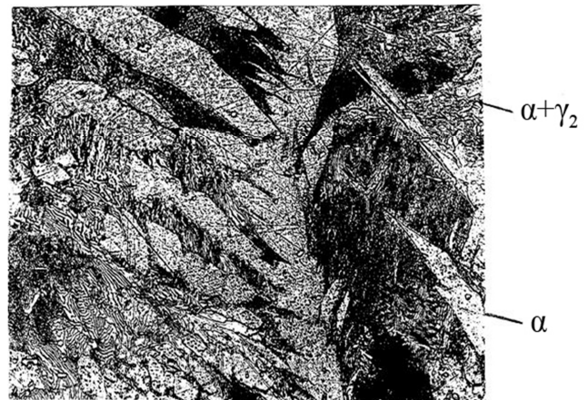
Figure 1. The microstructure of the diffusion layer (sample No. 1), X500.
