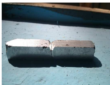
Figure 1(a). Percussion strength tested specimen.
