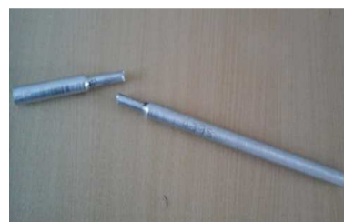
Figure 1(b). Tensile tested specimen.
