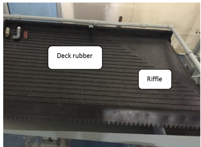
Figure 4. Results of Table/Deck Design and Installation of Rubber and Riffle Mats.
