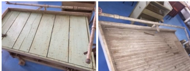
Figure 4. Results of Table/Deck Design and Installation of Rubber and Riffle Mats.
