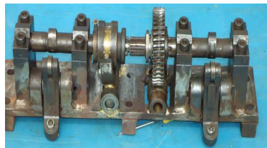
Figure 8. The mechanism for controlling cylinder deactivation.
