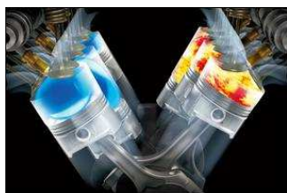
Figure 1. Cylinder deactivation for a 6 cylinder engine [1]
