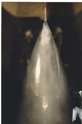
View n° 6. By increasing the incidence to 70°, the breakdown phenomenon of vortex structures becomes apparent, the flow of which, according to the incidence, swirl towards the apex of the give of revolution.
