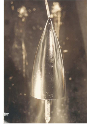
View n° 2. When the incidence is increased, the main vortices and the secondary vortex torque are now observed, the speed remaining constant. However, variation in the speed have no effect at all on the formation of vortex angle of 32^\circ
