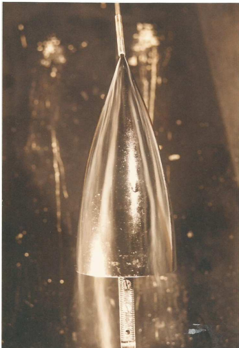
View n° 1. An angle incidence of 8^\circ ; the flow is uniform on the upper side of the wing. The boundary layer is observed but there is non flow separation as yet.
