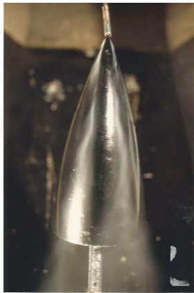
View n° 5. The formation of two vortex torques is detected, separated by an air corridor (a non-vortex passage) while the breakdown of the both main and secondary vortices begin. Angle of incidence of 55°.
