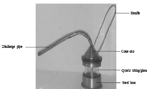
Fig 9. Improved Model of the Lantern Retort.
