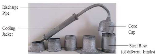
Fig 5. Components for the Retort Unit
