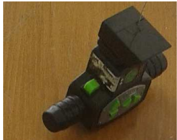
Fig. 9. Used radio controller type of solar submarine for near distance.
