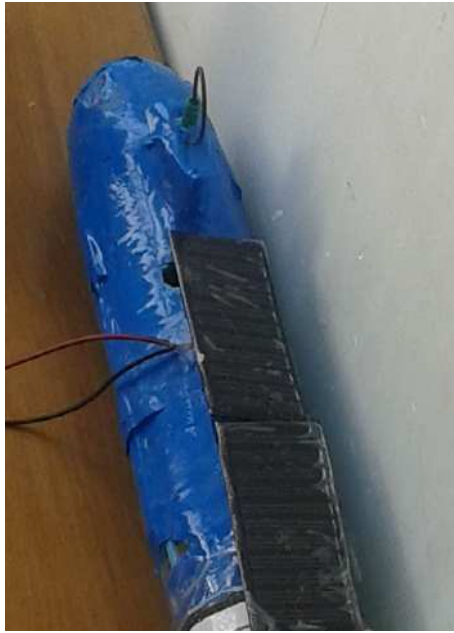
Fig. 3. Solar panels installed on submarine.
