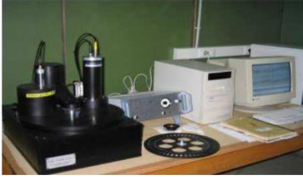
Figure 1. (photo). TL / OSL RISO-DA-15 reader at the Laboratory of Plasma at NCSR "Demokritos".
