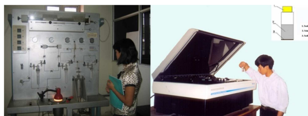
Figure 10. Practising benzene synthesis and measurement beta radioactivity in the Laboratory.
