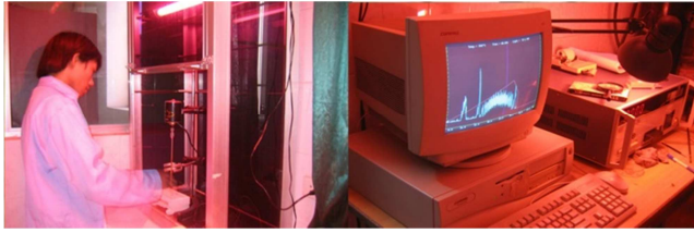
Figure 7. Treatment sample and measurement thermoluminescence in the Laboratory.
