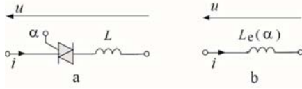
Figure 9. A thyristor switched inductor (a) and its equivalent inductance (b).
