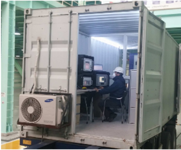
Fig. 1. The equipments of nondestructive test in 30kV generator stator windings.
