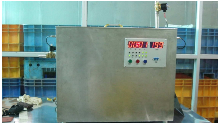
Figure 8. Ultrasonic processor made using the BLTs.
