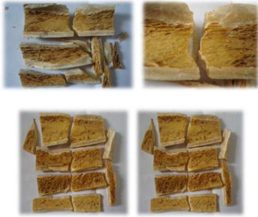
Fig. 10. Proximal and Distal regional (without crack) specimen subjected to impact load.
