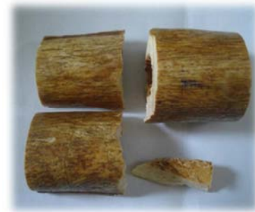
Fig. 8. With crack specimen subjected to impact load.
