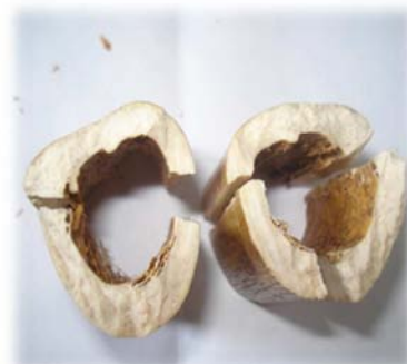
Fig. 9. a) Proximal regional and b) Distal regional (with crack) specimen subjected to impact load.
