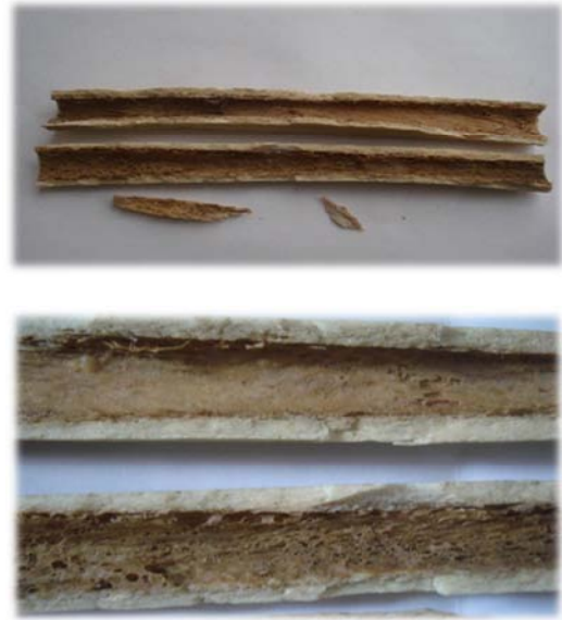
Fig. 15. With crack bending test specimen after test.
